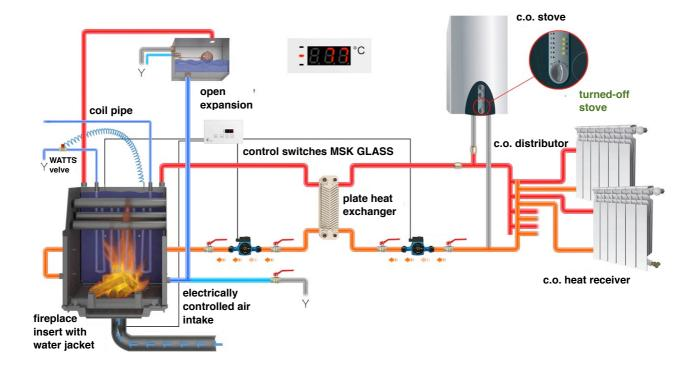
The BVTS thermal safety valve is used only in fireplaces with a water jacket and with the heating coil. It protects the water in the water jacket of the fireplace insert against boiling, e.g. in the case of a power failure when the circulation pumps stop working.
