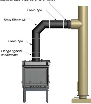
Transistion Steel Pipe Ceramic Chimney
