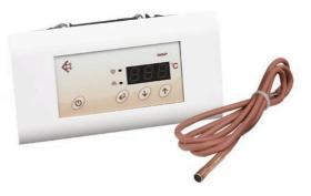
Apart from its basic functions, the controller also informs about the fact that the alarm temperature has been exceeded, protects the installation against freezing by automatically switching off the central heating pump if the temperature measured falls below 4°C and against self-activated switching from the stand-by mode after detecting an increase in the temperature of the liquid in the installation.
