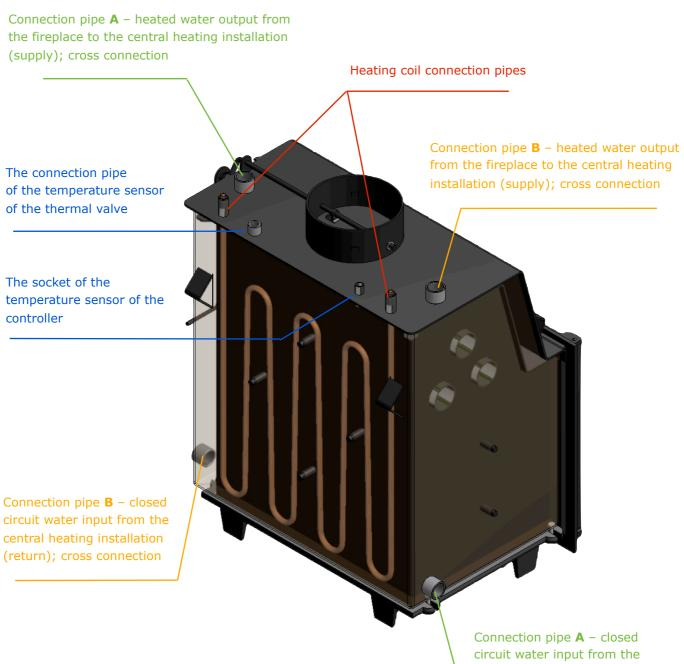
circuit water input from the central heating installation (return); cross connection
